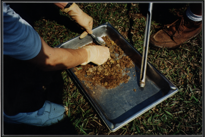
Plate 2.22: Removing a soil core from the sampler, and compositing ten separate cores from a given station.
